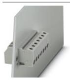
Panel feed-through terminal block, Connection method: Screw connection, Screw connection, Load current: 41 A, Cross section:  $0.2 \text{ mm}^2$  -  $6 \text{ mm}^2$ , AWG 24 - 10, Connection direction of the conductor to plug-in direction:  $0^{\circ}$ , Width: 8.1 mm, Color: gray
