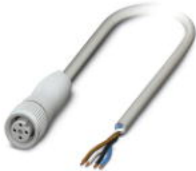
Sensor/Actuator cable, 4-position, PP-EPDM halogen-free, Gray RAL 7035. Free cable end, on Socket straight M12, A-coded, Cable length: 3 m, Hygienic design, with plastic knurl
